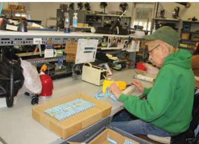
GLUING AND WELDING: Pam Mest glues and welds cells to make a battery pack.
