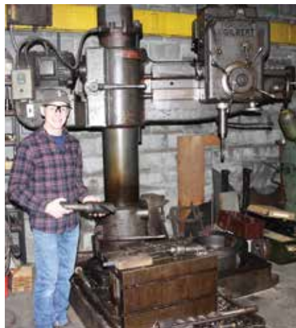
EQUIPMENT: This large drill press bit is used for making very large holes.
